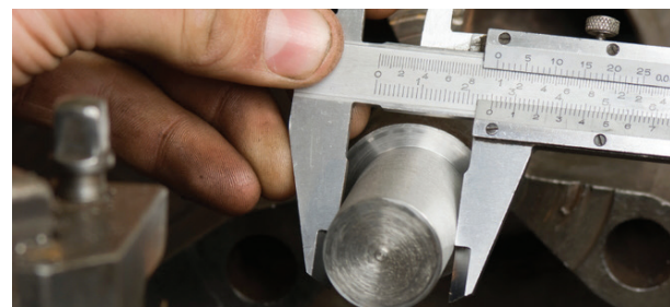
Figure 1.5 Measuring thickness of the cylinder using vernier caliper
