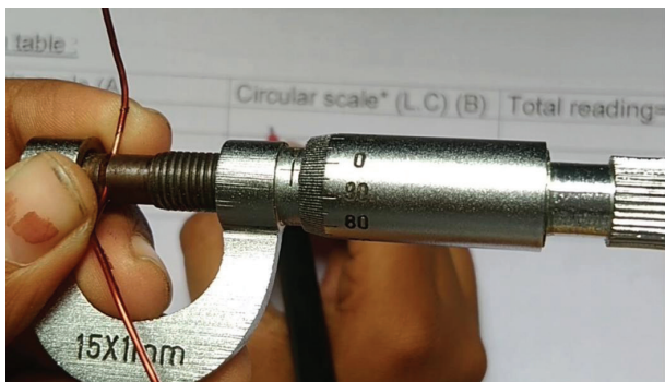
Figure 1.3 Measuring thickness of a given wire
